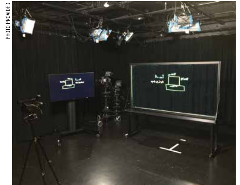
A digital camera reverses the image on the lightboard so images and text are easy to read on the video.
